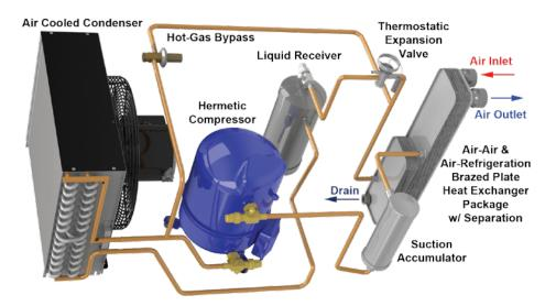
The expansion of the liquid causes the Freon to cool which is the equal and opposite reaction to the heat generated by compression. The cold Freon adsorbs the heat of the compressed air stream and evaporates to a gas. Any residual liquid is collected and evaporated in a suction accumulator prior to reentering the compressor before the process repeats.
