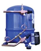
Heavy duty, industrial service piston type refrigeration compressor with proven durability that is designed to handle the fluctuating loads of a compressed air refrigeration dryer. The compressor is equipped with an oil sight glass to verify lubrication levels as well as proper gas return operating conditions. Rotolock service valves allow isolation as well as access to the refrigeration system that aids in the long term service and maintenance of a refrigeration dryer.
