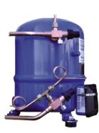
Heavy duty, industrial service piston type refrigeration compressor with proven durability that is designed to handle the fluctuating loads of a compressed air refrigeration dryer. The compressor is equipped with an oil sight glass to verify lubrication levels as well as proper gas return operating conditions. Rotolock service valves allow isolation as well as access to the refrigeration system that aids in the long term service and maintenance of a refrigeration dryer.
