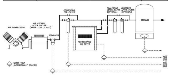
The pipe connection to the dryer should match the standard connection ports provided. The chart below is provided as a basic guide to size branch and header piping. It is recommended that shut-off valves with unions be installed at each port, with a valve bypass to permit isolation of the unit for servicing without interruption of plant air supply.
